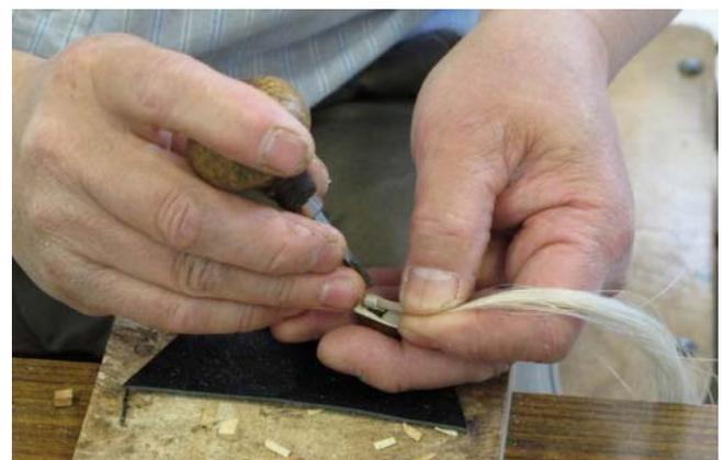
For the final steps, Jon secured the bow in his re-hairing jig: This holds the tip-end wedge and hair securely in place during the rest of the process.
