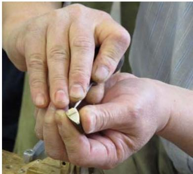
He did the same at the frog, slipping the metal ferrule off the thumb-rest, then removing the wedge and discarding the final bit of old hair. Now the bow was "bald" (see upper right picture).
