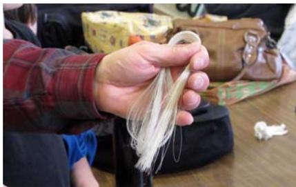
The hair is held in a "box" at each end of the bow under a wooden wedge. Jon used an awl to remove the wedge at the tip, releasing that stub-end of the old hair.
