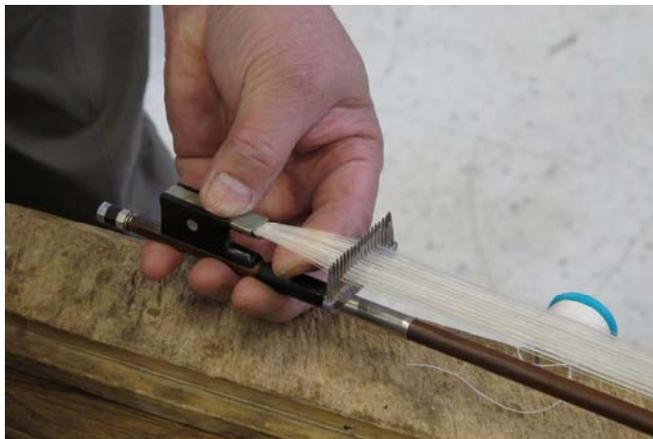
and cut those out. He noted in passing that the often-seen practice of yanking the end of a broken hair from the bow-tip risks dislodging the tip-end wedge – so he recommends cutting (or biting!) the hair off, instead.
